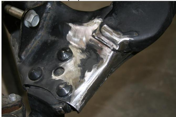
**Step 4:** Use a wire wheel or fine grit sanding disc to remove all paint and prep the surface for welding.
