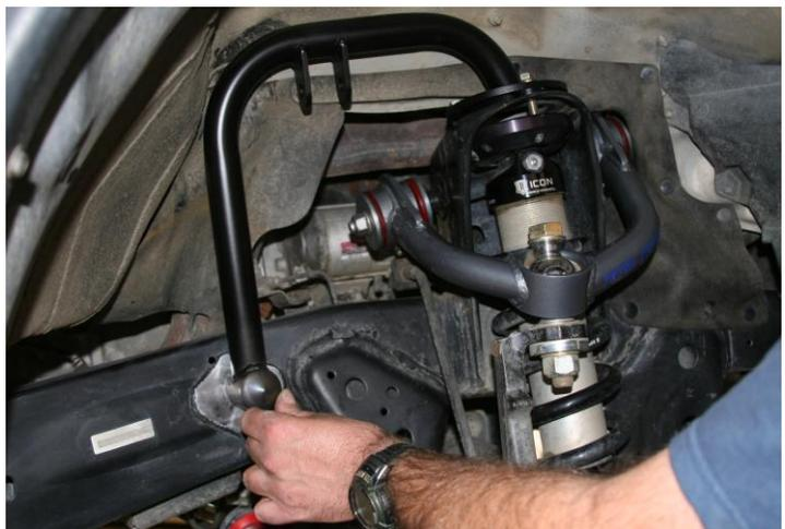
**Step 8:** Tack weld the diamond overlay onto side of frame. Then tack the main hoop to the 1 1/2" tube boss, then to the side of the frame. Complete the set up by tack welding the hoop to the circular mount. Leave these items only tack welded for now. (See Pic 1, Pic 2 & Pic 3)
