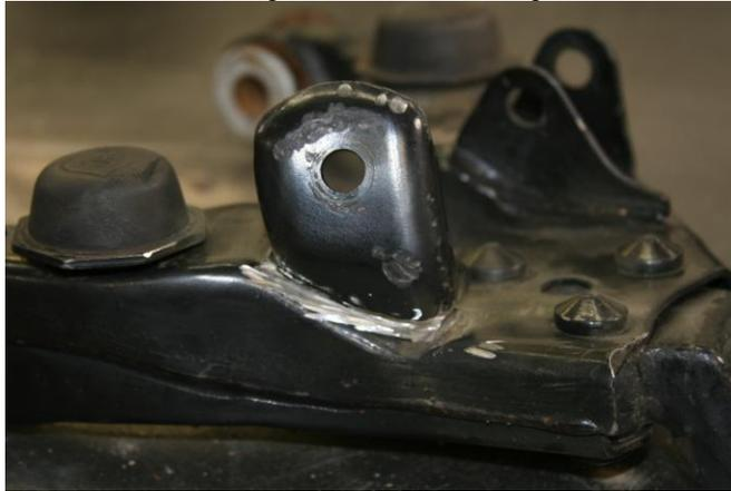
**Step 3:** Set lower shock mount onto the lower arm and line up the two notches in the shock mount with the rivet heads, this will set the location of the lower shock mount. Now trace around the entire perimeter of the mount top and underneath with a bright marker or silver pencil to mark the area in order to prep the surface.
