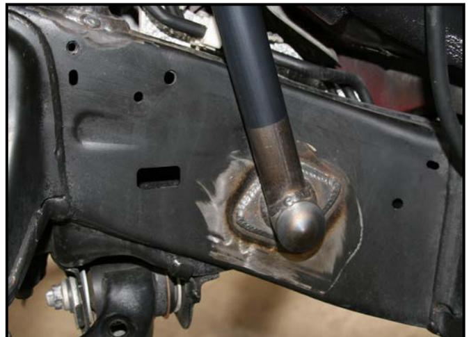
**Step 9:** With the 4 shock hoop bolts tightly in place, tack weld the two outer bosses to the coil bucket. This will assure that the shock hoop will not move when the shock bolts are removed in the future.
