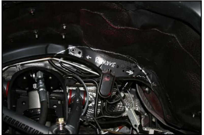
**Step 6:** Bolt the shock hoop to the top of the coil tower with new longer supplied 3/8" hardware. Snug all the hardware at this time.
