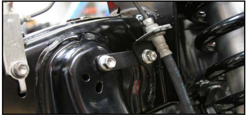
**Step 15:** Install the shocks on both sides with the supplied hardware and charge to manufactures recommended PSI.
