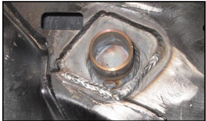
7. Then reinstall the hoop and weld it to the hoop boss (or boss to the frame depending on how you did it)
