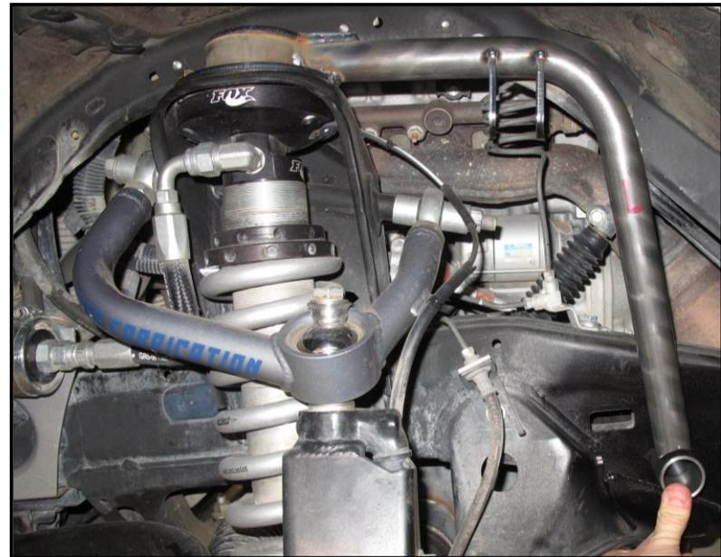
2. Mark on the side of the frame where the frame overlay plate and hoop boss will be welded. Then remove the hoop and remove the paint from the area where the overlay plate will be welded.
