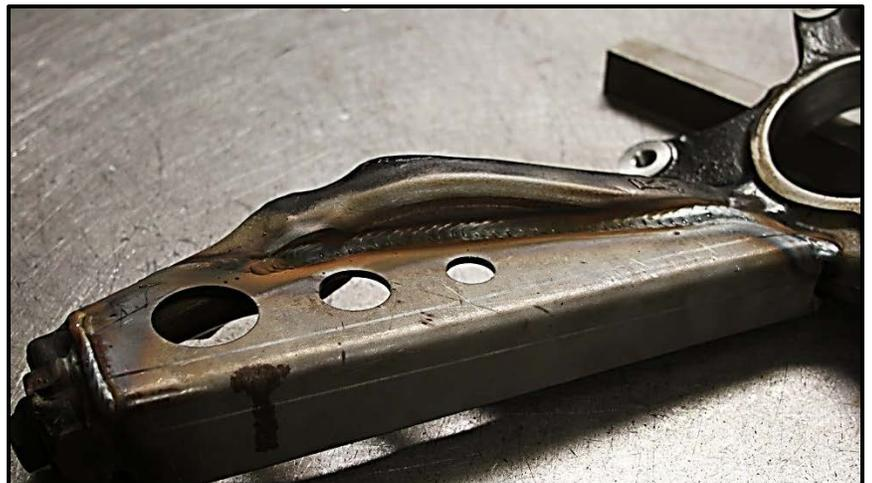
15. Paint the welded areas and new gusset itself. Re-install the upper ball-joint (95ft lb) (or 9/16" bolt 100ftlb), lower ball joint cradle, hub assembly, axle nut and dust cap, tie rod, rotor, caliper, and wheel speed sensors.
