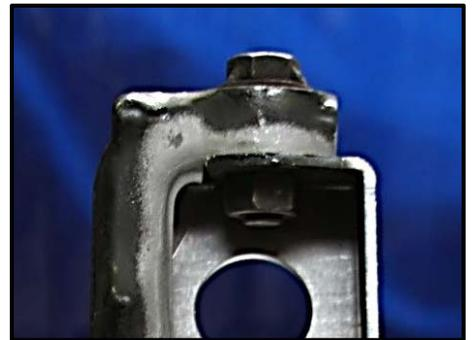
14. Weld along complete top and sides of the spindle, also weld the bend seam. Weld the lower portion of the spindle gusset closest to the hub on both sides in and out. (It is recommended to weld in moderation, do not overheat the spindle.) **\*\*Recommended: Weld some on one spindle, then move to the other spindle so you do not overheat one spindle.**
