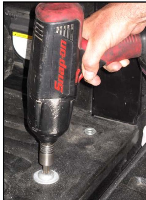
6. Set the new bracket in place, and install the provided  $7/16''$  bolt with the supplied washer on the top of the bracket and the factory washers where the stock tie down mount was underneath the bracket.
