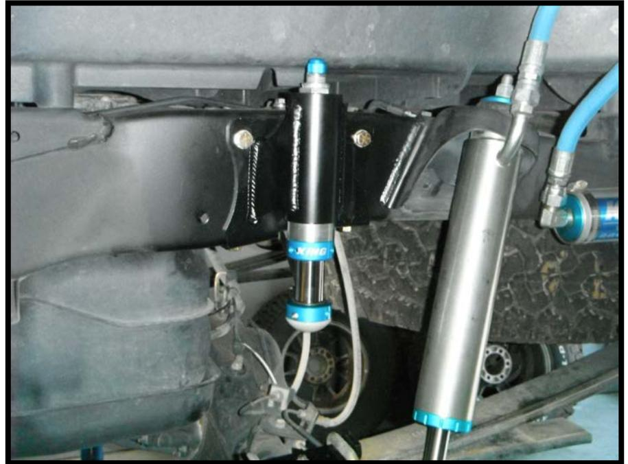
5. If installing Fox 2.0 bumps the bottom rib of the bed will need to be notched to clear the body of the bump stop.
