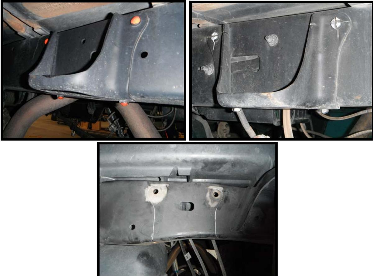
3. With a jack under the rear axle, remove the U-bolts and replace the factory rubber bump stop with the new bump stop strike plates. Remove and replace one side at a time and torque U-bolts to factory spec.
