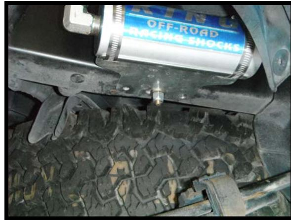
Suggested mounting location for driver's side reservoir. Mount the King reservoir bracket to existing hole in the bottom of the frame using the slotted center hole in bracket.
