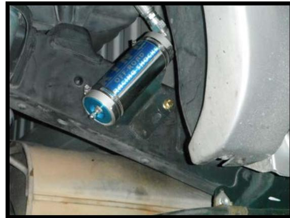
Passenger side suggested location. Mount bracket to existing hole in the side of the frame using the right hole in the bracket.
