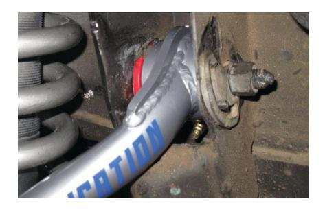
**Step 7**: Install the shock, and tighten the upper and lower bolts.
