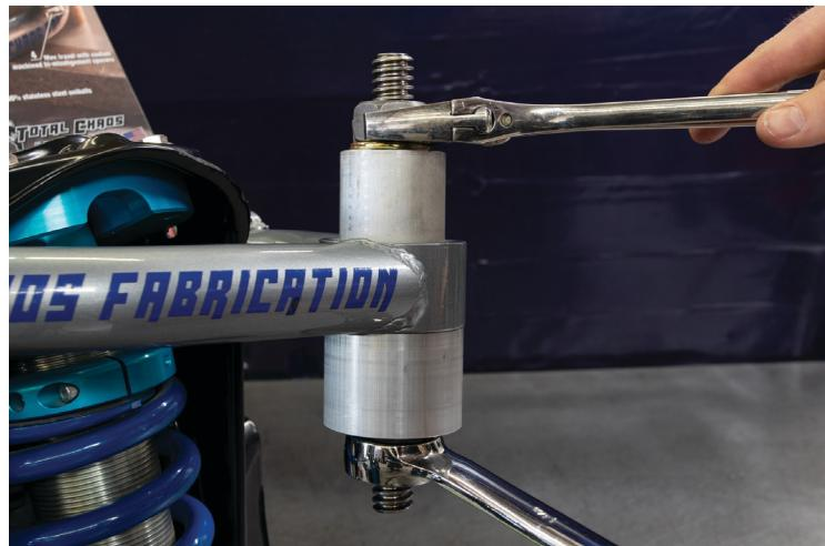
The small press tool cup will begin to push the uniball out of the bottom of the arm into the large press tool cup.
