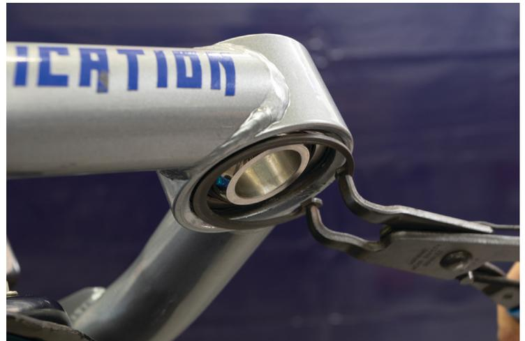
*NOTE: Make sure the snap ring gap is clocked towards the front or rear of the vehicle so it doesn't hinder the rotation of the misalignment spacers during the suspension cycle.*
