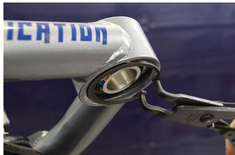
*NOTE: Make sure the snap ring gap is clocked towards the front or rear of the vehicle so it doesn't hinder the rotation of the misalignment spacers during the suspension cycle.*
