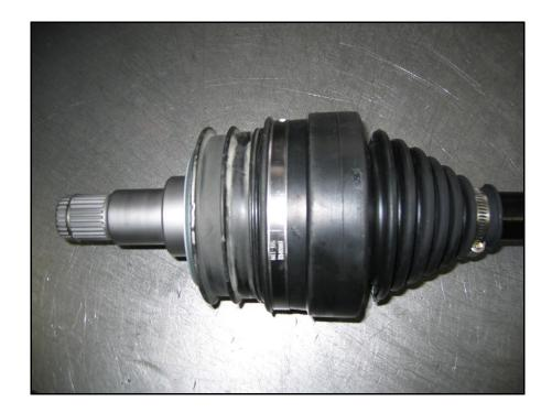
In order to remove the factory outer CV joint the stock axle shaft will need to be cut.
