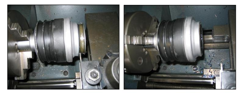
Flange for factory inner CV boot must be trimmed off to allow for full range of motion. New high angle inner CV boots (provided) will install as seen below:
