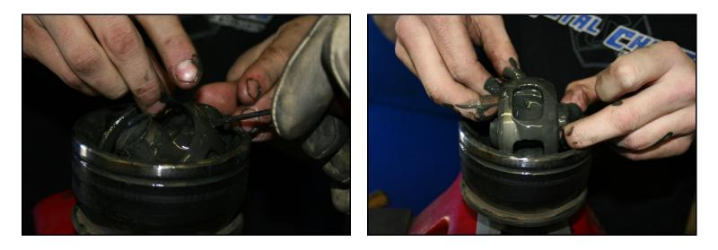
With the balls removed, the cage and star can be rotated and removed. Press the stub of the axle out enough to remove the snap ring and then remove the stub. Re-assemble the outer CV (star, cage, and balls). Insert the new shafts with the new snap rings installed into the outer CV joint. Install boots and inner CV joint (this is a good time to use new CV grease as well as new outer CV boots from Toyota), then install into the vehicle.
