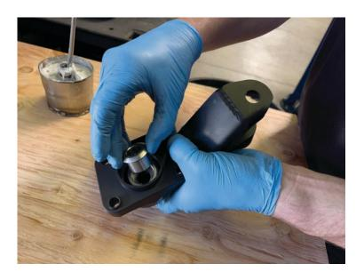
The tall misalignment spacer with a built in tapered adapter goes in the bottom of the uniball.
