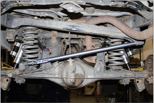
NOTE: On 2010+ models the lower link bracket on the axle will need to be modified to access the zerk fitting, see pics below:
