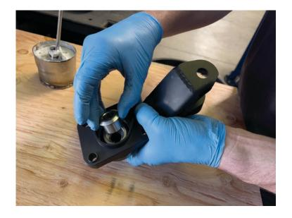
The tall misalignment spacer with a built in tapered adapter goes in the bottom of the uniball.
