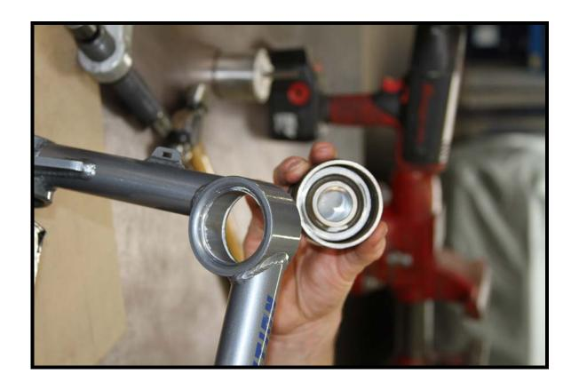
4. With the old uniball out, wipe down the inside of the uniball cup and apply a new layer of antiseize. This will aid in the installation of the new uniball as well as make any future removal/replace ment much easier.
