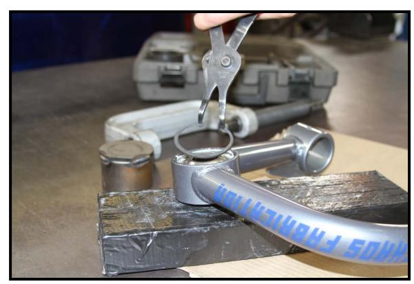
2. Position the tools for uniball removal. The smaller diameter tool will press on the uniball race from the top side of the control arm while the larger diameter tool will rest on the bottom side of the uniball cup to catch the ball once it is free.
