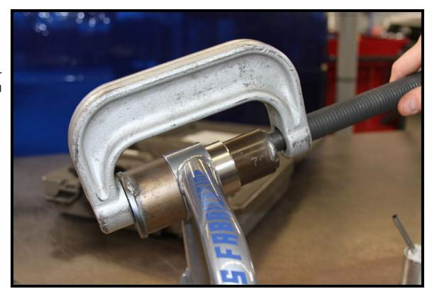
6. If the uniball gets crooked as it is pressed it, remove the balljoint press and use a hammer and block of wood to straighten it out.
