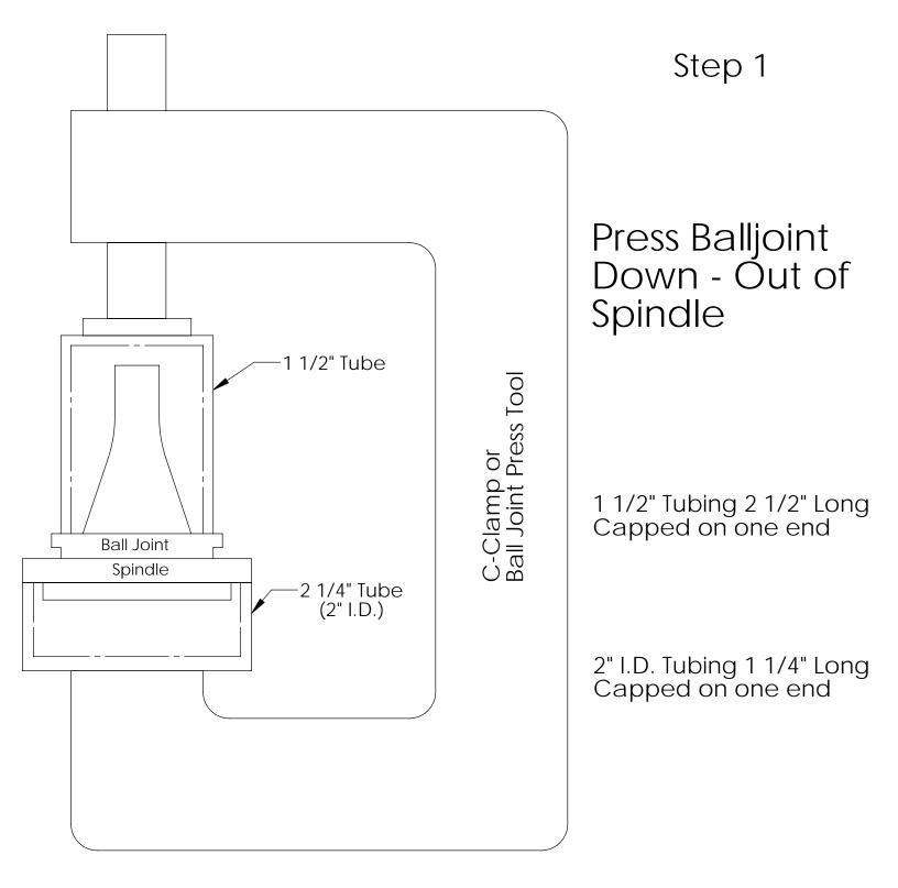
Remove ball joint castle nut, boot and snap ring. Press ball joint down and out of spindle using tubing.
