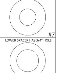
WHEN ROTATING THE UCA DOWN TO MATE UP TO THE SPINDLE, ENSURE THE HI-MISALIGNMENT SPACERS STAY FULLY SEATED IN THE UNIBALL. DAMAGE MAY OCCUR IF THEY ARE ONLY PARTIALLY SEATED WHILE THE UNIBALL BOLT IS BEING TIGHTENED.
