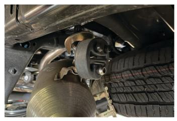
Ratchet strap shown connected to exhaust hanger.
