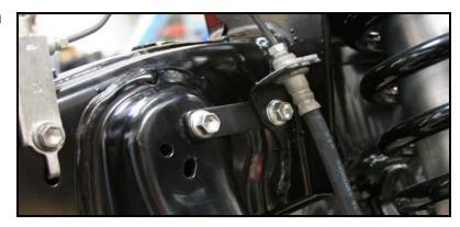
Step 15: Install the shocks on both sides with the supplied hardware and charge to manufactures recommended PSI.
