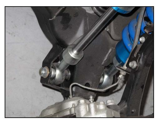
**Step 12:** Reservoir clamp mounts (weld on) with the shock hoop welded in place bolt in the secondary shock to establish reservoir clearance. Check tires when fully turned each way to make sure reservoir clears the tire. Tack the clamps into place. Remove shock and reservoirs weld clamps to the shock hoop. (See photos)
