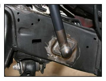
**Step 9**: With the 4 shock hoop bolts tightly in place, tack weld the two outer bosses to the coil bucket. This will assure that the shock hoop will not move when the shock bolts are removed in the future.
