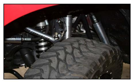
**Step 13:** After welding we recommend that you spray paint as much of the hoop and frame as possible before re-installing the secondary shocks.
