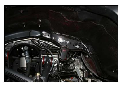
Step 7: Place the rear portion of the shock hoop up against the frame, holding the stand off up to it.
