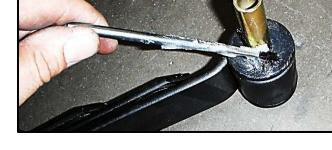
5. Mount new shackles to upper shackle mount. With the springs under the rear end mount the new springs to the new shackles and snug bolts. (note: shackles angle back, see photo)
