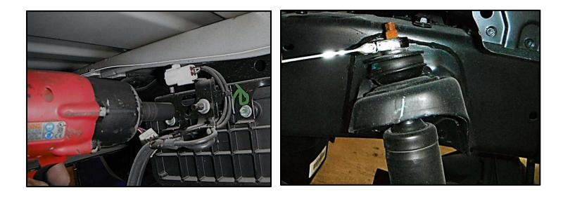
4. Lubricate the spring bushings as well as the inside of the leaf springs then mount the springs to the front spring hanger and snug bolt.
