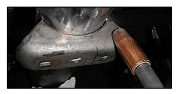
15. Once axle is cool, paint the new perches and re install the Ubolt s and U-bolt plates and tighten.
