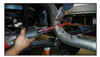
3. Once the truck is on jack stands remove rear tires, rear shocks, rear springs, U-bolts shackles (support the axle housing with two more jack stands before removing springs, U-bolts and shackles), rear bumper, factory tow hitch, rear rubber brake lines, and cut exhaust. Also move parking brake brackets and ABS wiring out of the way.
