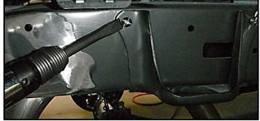
an air hammer to punch them through the frame. Once finished, clean and paint the frame to prevent rust behind the new bracket. (driver's side, remove nut in the center of the bump mount on the frame and zip tie the electrical box on the inside of the frame).
