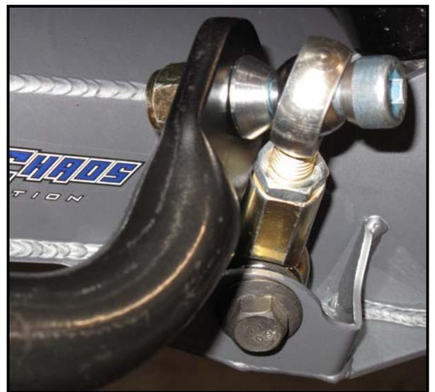
7. The heim joint angles are maxed out when the vehicle is at full droop they are not bound, just maxed out; do not be concerned about damage to the bolt or heim joint.
