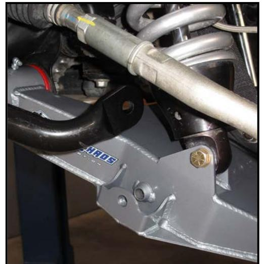
5. When holding the pre-set sway bar links up to the lower control arm and sway bay it will be obvious which links are left and right. Install the link (as shown) and install the supplied 14mm flange head bolt and nut. Using an 18mm wrench on the bolt head and a 21mm wrench on the nut, tighten the bolt (101ft-lb).
