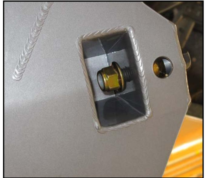
6. Install the supplied chamfered head Allen bolt through the sway bar link, supplied spacer, and sway bar, then spin on the supplied flange nut. Use a 12mm Allen wrench and a 21mm wrench to tighten the Allen bolt (101ft-lb).
