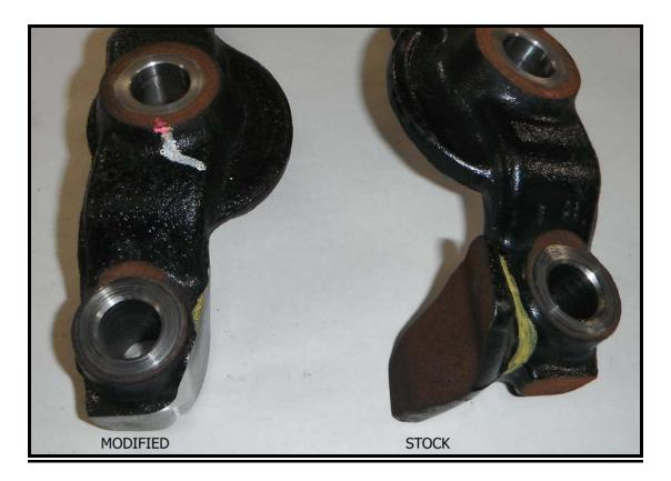
Steering stop must be trimmed off of the lower ball joint cradle or severe damage to the new lower control arm will result. Some contact may remain at full lock steering.
