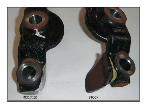
Steering stop must be trimmed off of the lower ball joint cradle or severe damage to the new lower control arm will result. Some contact may remain at full lock steering.
