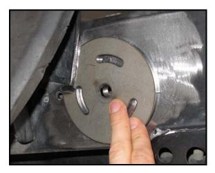
6. Using the supplied ½" x 1 ½" bolts, bolt the large circle overlay with nut to the front of the hoop, and put the bolt through the rear of the hoop and the large overlay without nut on the rear of the hoop making sure the overlay doesn't interfere with the bump stop bracket.
