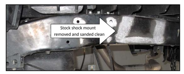
3. Next locate the front rectangle hole on the side of the frame, as well as the rear round hole just in front of the bump stop mount, and clean off the paint around both holes.
