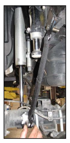
14. After tacking all limit strap tabs in place. Droop out the suspension and make sure that when fully extended, the limit strap is tight and the shock shows less than 10" of shaft.
