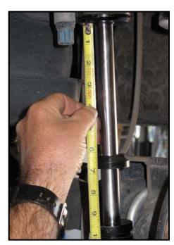
13. With the shock shaft only showing 9 ½", attach the supplied lower limit strap mounts to the strap and swing them over to the axle. Once again the strap will be pulling at an angle, so you will have to angle the tabs on the rear axle. The tabs should be roughly 4" in from the rear hub.
