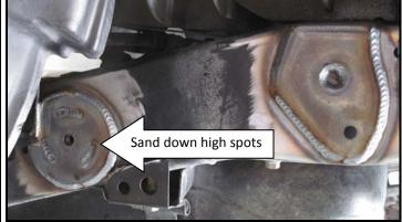
9. Once the frame is cool, bolt up the hoop using the supplied large frame backing plate on the back side of the frame on the rear hoop mount. Next hang the fully extended shock from the upper shock mount. Then bolt the supplied lower shock mount to the shock. Make sure the rear suspension is fully drooped, and swing the lower shock mount against the axle, making sure that the outer side of shock mount is 2 3/8" away from the axle flange, tack weld in place.
