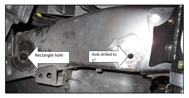
4. Using a drill bit or uni-bit, drill out the round hole ½".
