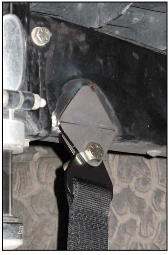
12.Next, with all the shock mounts securely tacked into place, jack up the suspension so that the shaft only shows 9 ½" of stroke.
