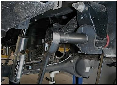
10) Remove the front spring hanger bolts. Now remove the leaf springs.
