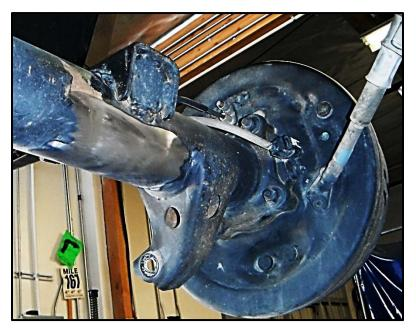
16) One spring at a time, use a jack under the center pin and jack up the spring until the shackle is above the rear shackle mount, then pull the leaf spring down until the shackle hole lines up with the frame mount hole and install the bolt. (Repeat on other side, this is easiest with two people)
