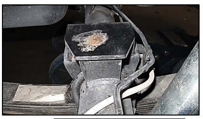
26) (When using stock rubber bump stops) Mark and trim some of the metal off of the bump stop so it fits on the new bump stop relocation pad.
