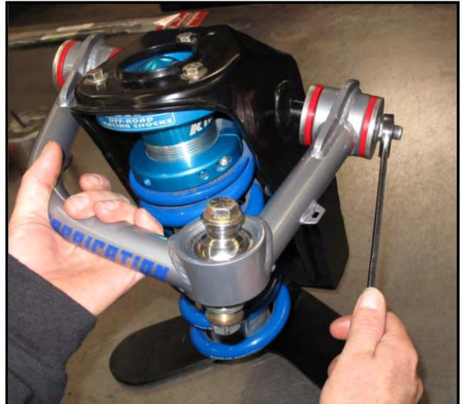
3. With the bolt loose, pump grease into the zerk fitting until you can see the excess grease bleed out from between the bushing “hat” and the plated end washer.
