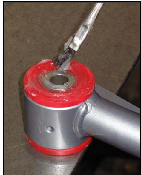
6. When installing the zerk fittings, it may be necessary to use a knife or sharp object to clean out the top of the threaded hole so the 1/4"-28 NTP threads will catch. When tightening the zerk, **DO NOT** try and tighten the zerk to the bottom of the thread. It is only necessary to turn the zerk until it gets snug. Then rotate as far as necessary to make the fitting accessible for a grease gun.
