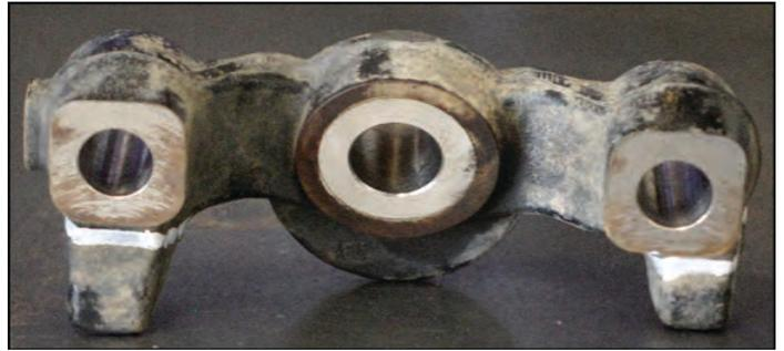
Cut the steering stops off of the Ball Joint cradle using either a band saw, hack saw, reciprocating saw, or a disc cutter.
