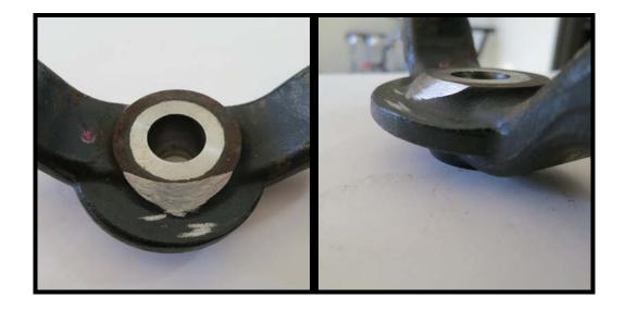
Bump stop spacer welded on and painted, reinstall the factory rubber bump stop into the threaded hole in the spacer.
