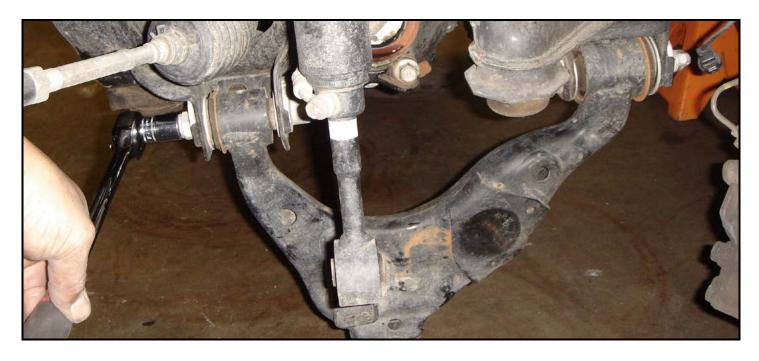
**Step 9: (Prep, Weld and Brake line removal and install and cradle prep)** With the lower arms removed it is highly recommended to clean and weld the outsides of the lower cam tabs. (This will insure that they will not bend. Total Chaos also offers replacement lower cam tab gussets part #'s 59860, 59860-10fj, 59960) If using the factory bump stops remove them from the
