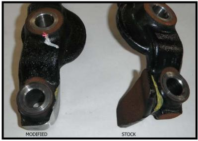
The area where the lower hi-misalignment spacer mounts to the ball joint cradle will also need to be modified. Grind the cradle as shown to properly clearance it for the lower control arm at full bump.
