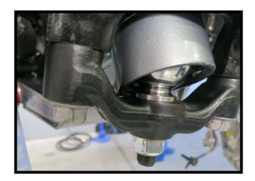
**Step 10: (Installing the lower control arm)** Before installing lower control arms you may need to bend lower arm tabs out slightly for easier fitment. With the welded areas painted (cam adjusters.) Grease the bushing face and tab face before installing arm into tabs. Use the factory hardware, center the alignment cams and snug down all at this time.
