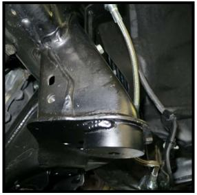
Cycle the suspension once this has been modified and the bump stop spacers have been installed to check for clearance.
