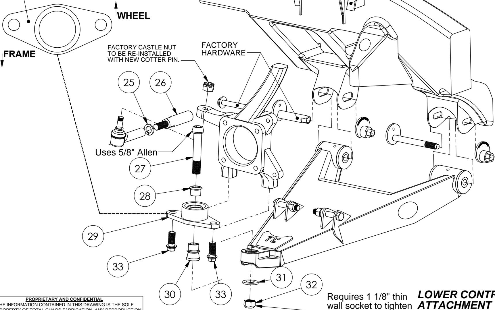
FACTORY CASTLE NUT TO BE RE-INSTALLED WITH NEW COTTER PIN.
