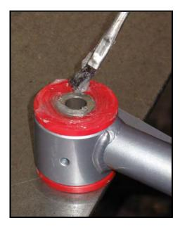
6. When installing the zerk fittings, it may be necessary to use a knife or sharp object to clean out the top of the threaded hole so the ¼"-28 NTP threads will catch. When tightening the zerk, DO <u>NOT</u> try and tighten the zerk to the bottom of the thread. It is only necessary to turn the zerk until it gets snug. Then rotate as far as necessary to make the fitting accessible for a grease gun.
