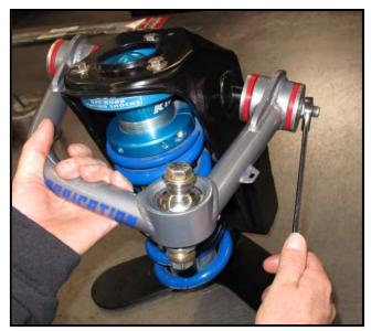
With the bolt loose, pump grease into the zerk fitting until you can see the excess grease bleed out from between the bushing "hat" and the plated end washer.
