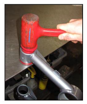
With the bushings installed in the control arm, generously apply grease to the inner diameter of the bushings trying to fill the bushing grooves completely with grease.
