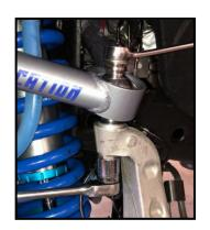
10. Use the stock bolt and supplied 6mm nut to attach the ABS bracket to the mount on the upper control arm (after flattening the tab from step 2). After this step your install is complete (image shown is 3.0 King Coil over). Re-check all hardware for tightness, reinstall the wheels and have a certified shop perform an
