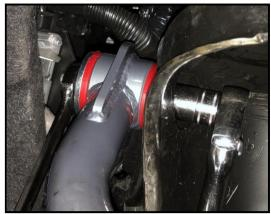
9. With the pivot bolts tight, re install the shock, then swing the UCA down and connect the uni-ball to the control arm using the supplied 9/16" hardware. Once the misalignments are seated with the tapered adapter and the bolt is installed, tighten the bolt using a 13/16" and a 7/8" wrench.
