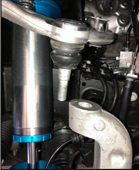
2. Remove the bolt (10mm) that holds the ABS wire bracket to the spindle. Then use a pair of pliers to flatten the bent over tab on the bracket.
