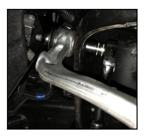
5. On the rear of the coil bucket there is a tab the appears to be used for the assembly line to hold the upper arm in place. This tab is no longer needed and can be easily broken off using a pair of channel locks bending it back and forth a couple of times.
