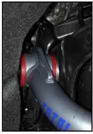
8. Place the remaining two washers and factory nuts on the outside of the bushings, then use a 21mm wrench to tighten the pivot bolts.
