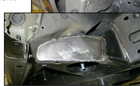
The plate, as well as the body mount may take some additional trimming, and bending/forming to get it to fit perfectly. Once it is fit, tack it in place and turn your tires back and forth to make sure the clearance is sufficient. If so, weld the new plate to the body mount.
