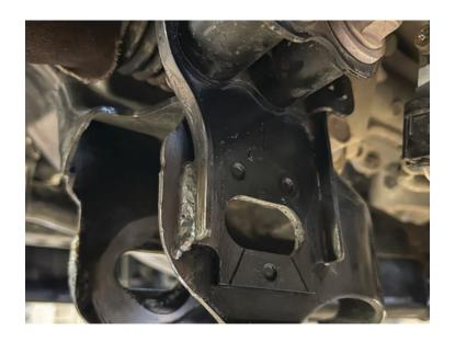
The following steps will cover the remaining six cam tabs with removal of the stock plates and installation of the TC cam tab plates & tabs.
