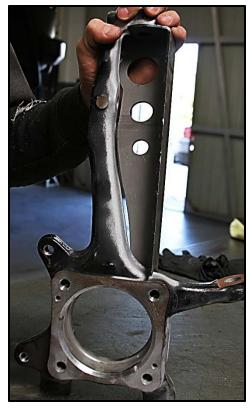
13. Once the paint is removed hold the knuckle up to the upper control arm and insert the ball joint (or 9/16" bolt) through the knuckle and the spindle gusset plate. Tighten the ball joint nut to secure the gusset plate in place and tack the gusset to the spindle in numerous locations. Then remove the spindle from the upper control arm.
