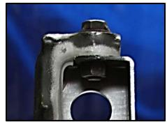
14. Weld along complete top and sides of the spindle, also weld the bend seam. Weld the lower portion of the spindle gusset closest to the hub on both sides in and out. (It is recommended to weld in moderation, do not overheat the spindle.) \*\*Recommended: Weld some on one spindle, then move to to the other spindle so you do not overheat one spindle.
