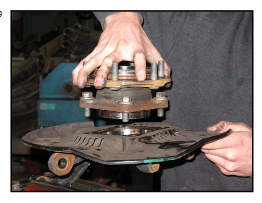
**STEP 2:** Unbolt and remove the ABS Sensor from the Spindle.
