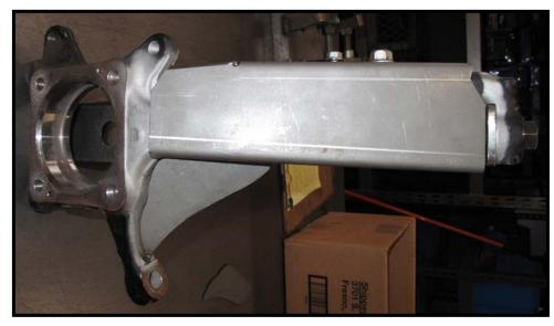
**STEP 6:** Start by welding the 10 gauge gusset pieces to each other, and then weld the gusset to the factory spindle. MIG welding is preferred but TIG can also be used.
