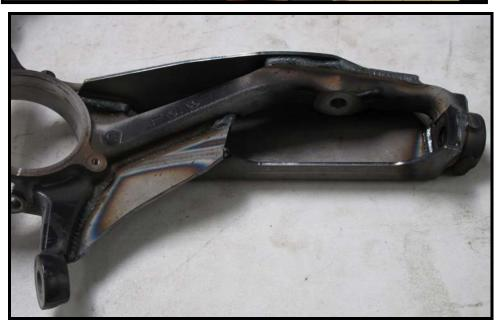
**STEP 7:** Paint after spindle has cooled. Mask off the bearing area and all threaded holes prior to painting.
