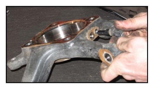
**STEP 3:** Remove the rear seal with a thin chisel or scraper. Replace if damaged (4wd models only).
