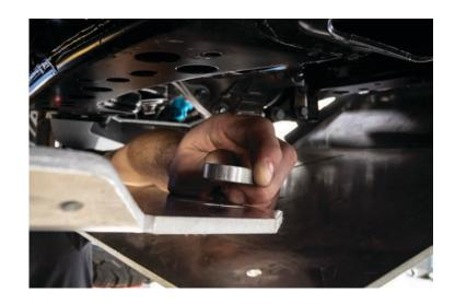
The skid plates should be stacked in the following order from bottom to top; front skid, rear skid, short spacer then frame.
