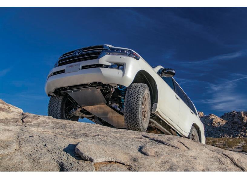
**COMPONENT: SKID PLATE AND BELLY PAN**
