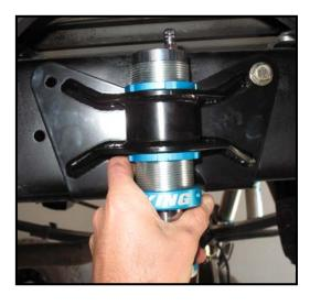
8. With the bump stop installed in the bracket, adjust the lock rings so that the distance between the bottom of the bump stop body and the bottom of the bump stop bracket is 2".
