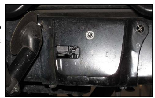
broken off, remove the bump stop bracket using a hammer.
