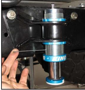
10. Support the rear axle with a jack or jack stand and remove the U-bolts that hold down the stock rubber bump stop, then remove the stock bump stop.
