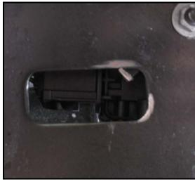
6. Also on the driver's side there is a stud and nut that sticks through the frame. The extra thread that sticks through the nut needs to be sanded flush with the top of the nut. Once finished with the sanding, spray paint any raw metal to protect the frame from rust
