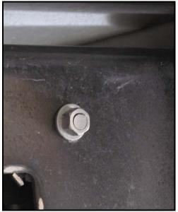
7. Install the bump stop into the bracket, and the bracket to the frame using the 7/16" hardware. Once all the hardware is installed tighten all the 7/16" bolts and nuts (52 ft-lb).
