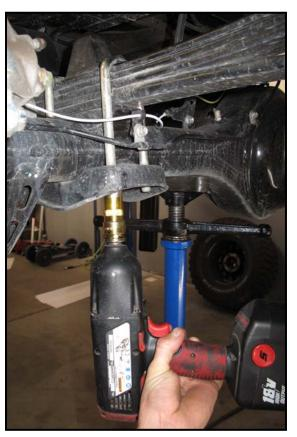
11. Set the new bump stop strike pad on top of the leaf spring lining up the hole in the bracket with the leaf spring center pin. Set the U-bolts over the new strike pad, then re-tighten the U-bolts (85 ft-lb)
