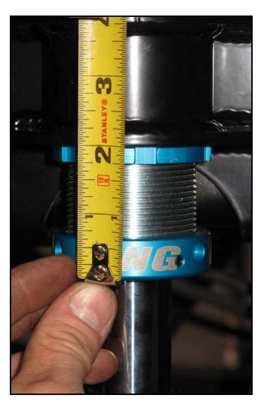
9. Once the bump height is adjusted correctly, use a spanner (or hammer and punch) to lock down the lock rings, as well as the 5/64" set screws on the top and bottom rings.
