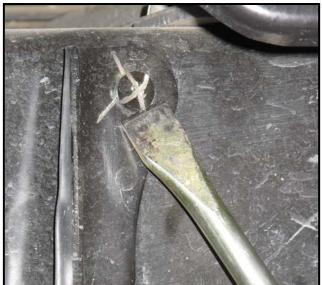
4. Sand down the left over rivets flat with the frame, then use an air hammer with a punch bit (or a hammer and punch) to push out the remaining rivet.
