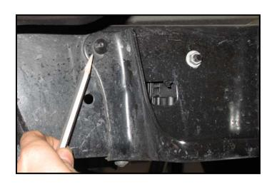
3. Use a disk cutter and cut an X in all four rivets. Then use an air hammer with a chisel bit (you can also use a hammer and chisel) to break off the heads of all four rivets.
