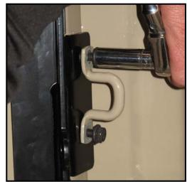
5. Thread the bed hold down bolt through the bed stiffener but do not tighten.
