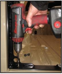
8. Insert and tighten the supplied 5/16" bolt, washers and nut in the bottom bed hole using a 1/2" wrench and socket, then drill the bottom hole in the bedside.
