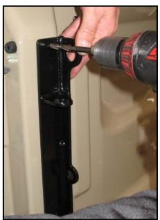
10. Insert and tighten the supplied 5/16" bolt, washers and nut in the top bedside hole using a 1/2" wrench and socket. While tightening this bolt you will see the previously mentioned gap disappear. Also tighten the stock tie down bracket using a 13mm wrench.
