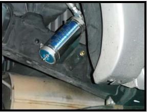
Passenger side suggested location. Mount bracket to existing hole in the side of the frame using the right hole in the bracket.
