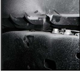
**6.** For vehicles equipped with King 2.5" Remote Reservoir Shocks you will need to relocate the reservoir mounting location using the supplied 3/8" hardware.
