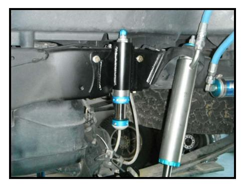
**5.** If installing Fox 2.0 bumps the bottom rib of the bed will need to be notched to clear the body of the bump stop.
