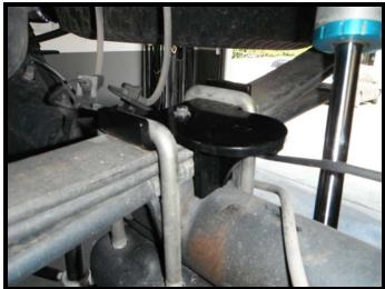
4. Install air bump into mounting bracket and bolt onto the frame using the supplied 7/16" hardware (in some cases you will need to ream out the holes in the frame to insert the hardware).
