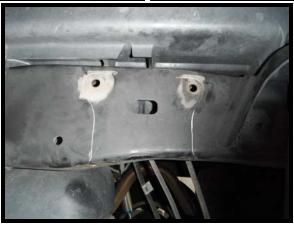
**3.** With a jack under the rear axle, remove the U-bolts and replace the factory rubber bump stop with the new bump stop strike plates. Remove and replace one side at a time and torque U-bolts to factory spec.
