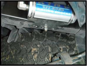
Suggested mounting location for driver's side reservoir. Mount the King reservoir bracket to existing hole in the bottom of the frame using the slotted center hole in bracket.
