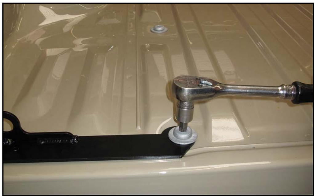
12. Make sure all the hardware is tight and re install the tail light using a T-30 Torx.
