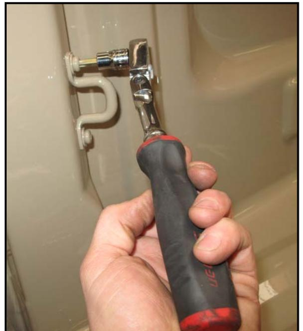
2. Use a T-30 Torx bit to remove both tail light bolts, then remove the tail light (pull the tail light out towards the side of the vehicle being careful to not break the plastic clips).
