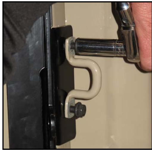
5. Thread the bed hold down bolt through the bed stiffener but do not tighten.
