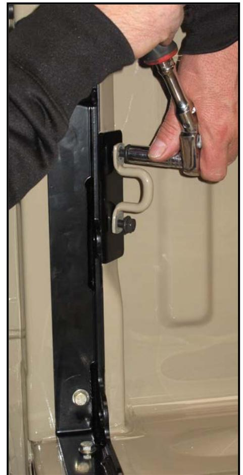
11. Use a T-55 Torx bit to tighten the bed hold down bolt.
