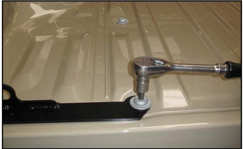
6. There will be a slight gap between the bed stiffener and the bed, this gap will cinch up when all the bolts are tight.
