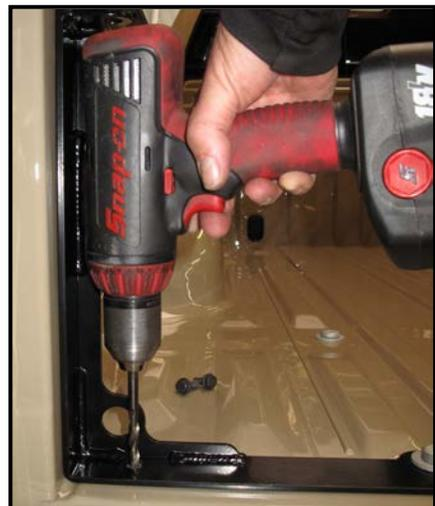
8. Insert and tighten the supplied 5/16" bolt, washers and nut in the bottom bed hole using a 1/2" wrench and socket, then drill the bottom hole in the bedside.
