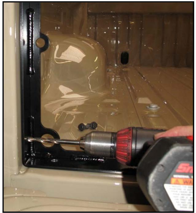
9. Insert and tighten the supplied 5/16" bolt, washers and nut in the bottom bedside hole using a 1/2" wrench and socket, then drill the top hole in the bedside.
