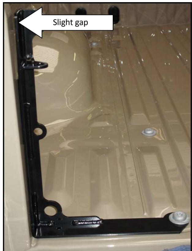
7. With the bracket in place, use a 5/16" drill bit and drill the bottom hole on the floor of the bed.
