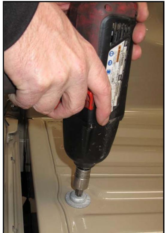
4. Put the new bed stiffener in place and install the stock tie down bracket with the supplied 8mm bolt using a 13mm wrench or socket. Do not fully tighten the bolts.
