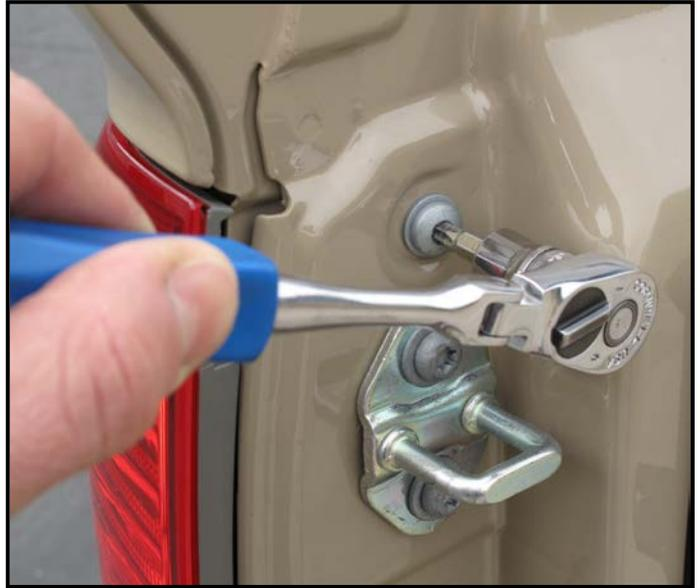
3. Use a T-55 Torx bit to remove the bed hold down bolt.
