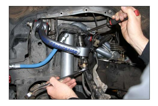
STEP 9: Set cams into position and tighten hardware (torque to 72 ft/lbs).
