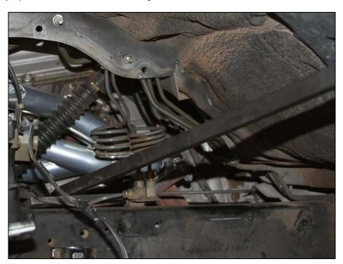
**STEP 4:** Using a good synthetic grease (preferable containing PTFE, TC recommends Superlube) assemble the new UCA's. Press in the new polyurethane bushings dry, then apply grease to the ID of the bushings. Next, press in the supplied metal inner sleeves. Finally, thread in the supplied ½"-28 zerk fittings. Do not over tighten as they are hollow and can snap off. Position the zerk fittings so they can be reached with a grease gun once the arms are installed on the vehicle.
