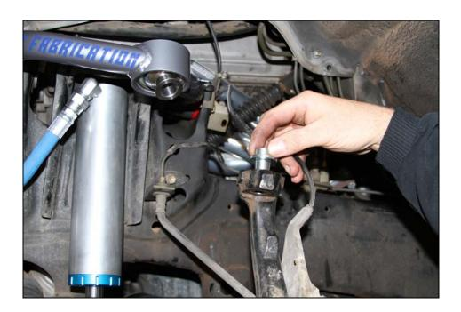
**STEP 8:** Pivot the upper control arm down until the lower hi-misalignment spacer in the uniball slides over the tapered spindle adapter sleeve. Coat the 9/16"-18 X 5" grade 8 bolt with a layer of anti-seize and insert through the assembly. Torque to 100 ft-lbs.
