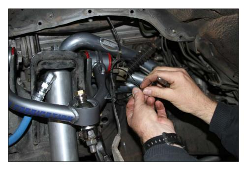
**STEP 11:** Double check that all hardware is properly tightened, then re-install the tires.
