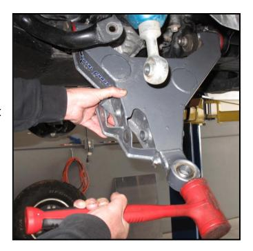
alignment cam bolts that connect the lower control arms to the frame.
